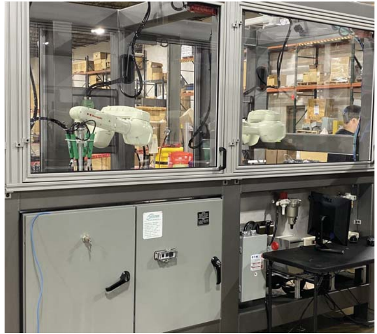
Two compact, high-speed Kawasaki RS007 robots pick product off the bag conveyor, and place them in boxes on a secondary conveyor below.
