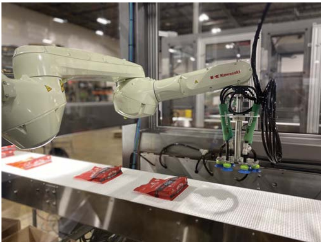
The Kawasaki RS007 robots are equipped with proprietary vacuum grippers designed specifically for picking bagged product.
